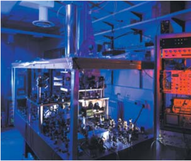
PRIMARY CLOCK for the U.S. is the NIST-F1 cesium fountain in Boulder, Colo. It is one of 200-odd clocks whose times are averaged to produce Coordinated Universal Time (UTC).
